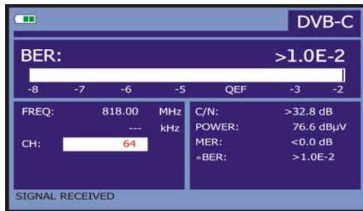
Figure 29.- DVB-C (QAM) signals BER measurement screen.
