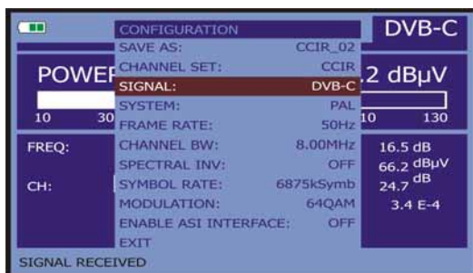
Figure 19.- Screen of measurement configuration (QAM signals).
